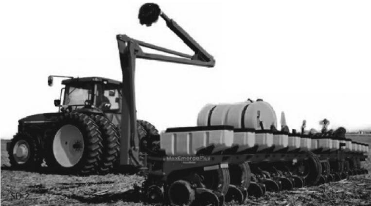
FIGURE 11.20 (See color insert.) Deere MaxEmergePlus planter. (Courtesy of John Deere Co., Moline, Illinois.)
